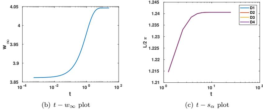
Figure 5: Time evolution of 4 elliptic regions with semi-axes  $a = 1.5$  and  $b = 1.0$ . The other parameters are  $R_\infty = 4$  and surface tension  $\sigma = 0.47$ . The system enters equilibrium at  $t_{eq} = 8.75$ . Centroids of the domains D1, D2, D3, and D4 are at  $(2, 0)$ ,  $(0, 2)$ ,  $(-2, 0)$ , and  $(0, -2)$  at  $t = 0$ , respectively.
