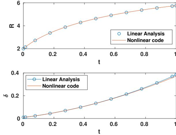
Figure 2: Comparison of results from the nonlinear simulation and the linear analysis for  $R(t)$  and  $\delta(t)$  against time. We choose  $\sigma = 0.47$ ,  $R_\infty = 10$ ,  $N = 1024$ , and  $\Delta t = 2 \times 10^{-3}$  to obtain the match between the two setups and the simulation are stopped when the linear analysis results starts to over-predict the nonlinear results at  $t_{\text{end}} = 1.0$ .
