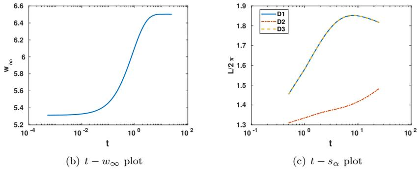
Figure 6: Time evolution of 3 elliptic regions with semi-axes  $a = 1.5$  and  $b = 1$ . We set  $R_\infty = 4$ . The system enters the equilibrium phase at  $t_c = 9.35$ . Centroids of the domains D1, D2, and D3 are at  $(2, 0)$ ,  $(0, 2)$ , and  $(-2, 0)$  at  $t = 0$ , respectively.
