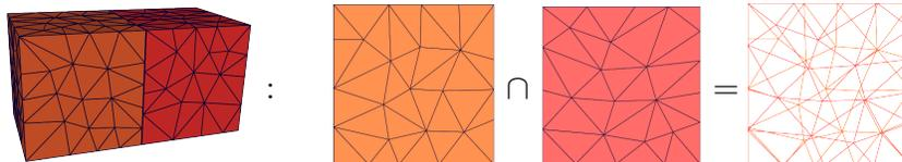
Figure 8: Coupling of two unrelated meshes via a merged grid: Intersecting the coupling patches yields a set of remote intersections, which can be used to evaluate the coupling conditions.
