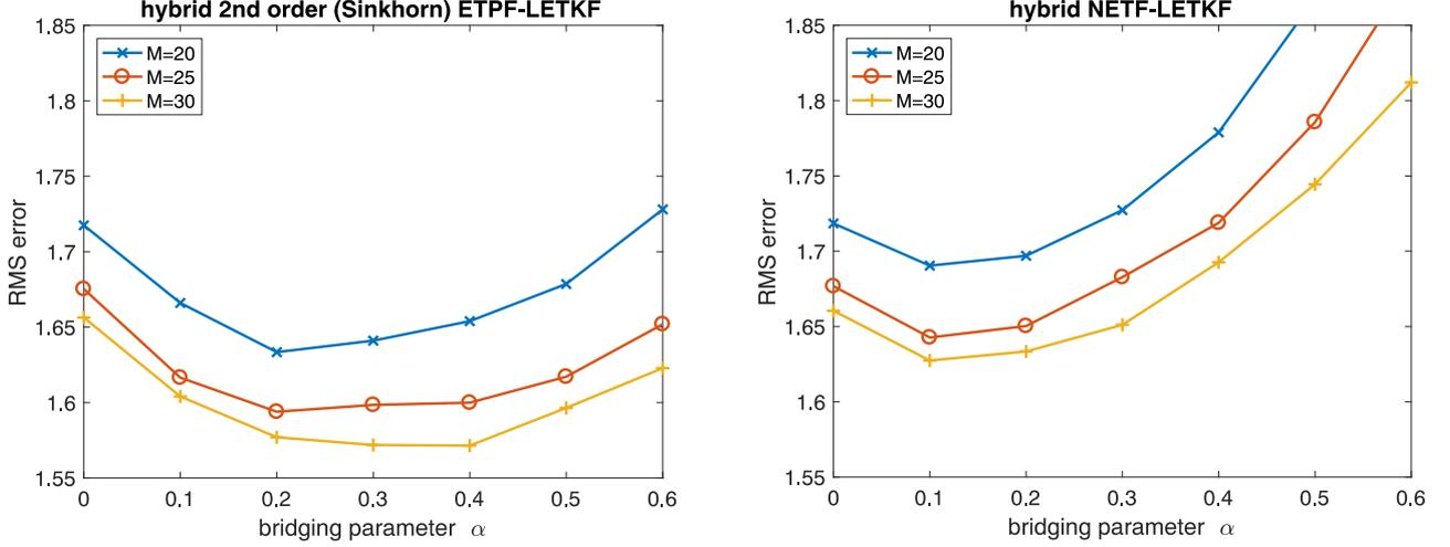
Figure 4: Second-order hybrid ETPF-LETKF with the optimal transport problem solved by the Sinkhorn approximation with  $\lambda = 10$  (left panel) and hybrid NETF-LETKF with the orthogonal matrix  $\mathbf{Q}$  at each grid point defined as in (35) (right panel) applied to the Lorenz-96 model. Time-averaged RMS errors are displayed as a function of the bridging parameter  $\alpha$ . The choice  $\alpha = 0$  corresponds to the LETKF
