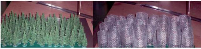
**Figure 5:** An artificial forest stand build by conventional tree models (left) and cylindrical wire frames (right).
