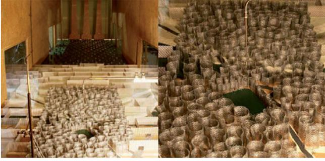
**Figure 4:** Left side: view along the wind tunnel. The Counihan vortex generators in the background are followed by the steel brackets and rectangular arranged roughness elements over the *S-Berg*, and, finally, the site model in the foreground. Right side: a close-up of the site model.
